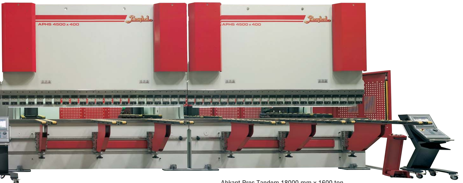
Abkant Pres Tandem 18000 mm x 1600 ton Press Brake Tandem 18000 mm x 1600 tons
