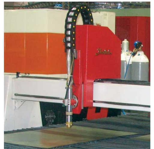
40 mm ye kadar High definition plazma ile donatılmış makine modeli. High definition work type model for plasma cutting up to 40 mm.
