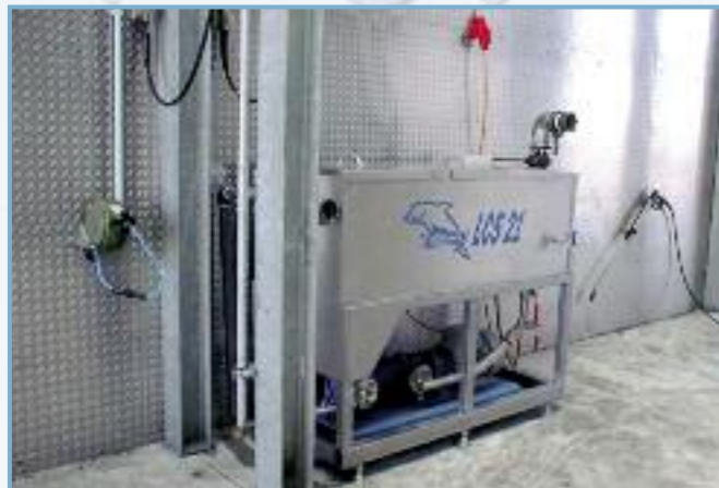
Close loop cleaning system for latex, dispersion or racine.
