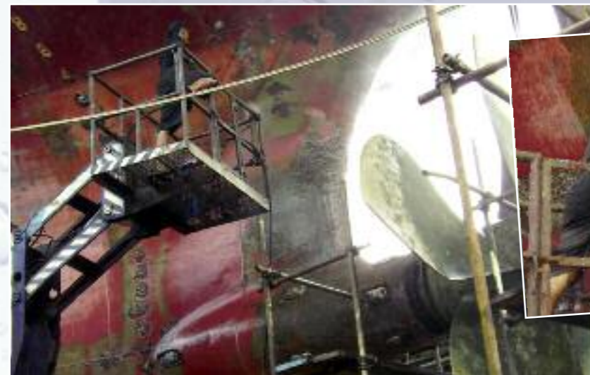
Application of a 400 bar high pressure cleaner in a chinese dry-dock.
