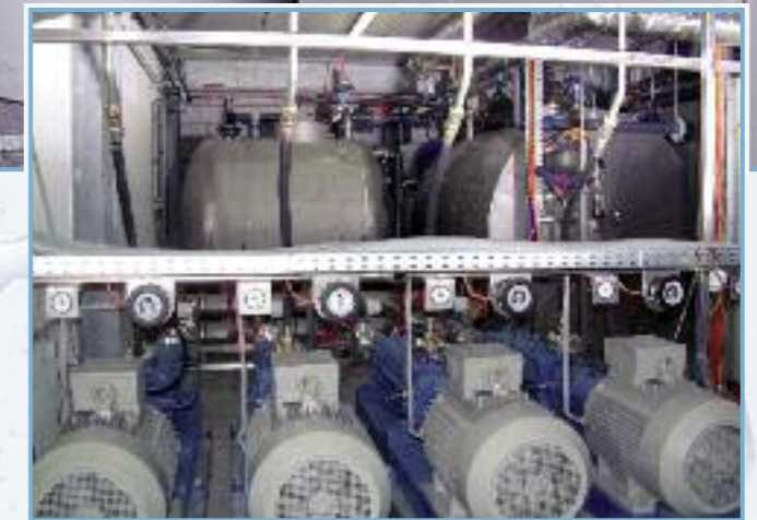
Pump technology of a 4 bay tank cleaning system, being able to wash up to 250 compartments a day.
