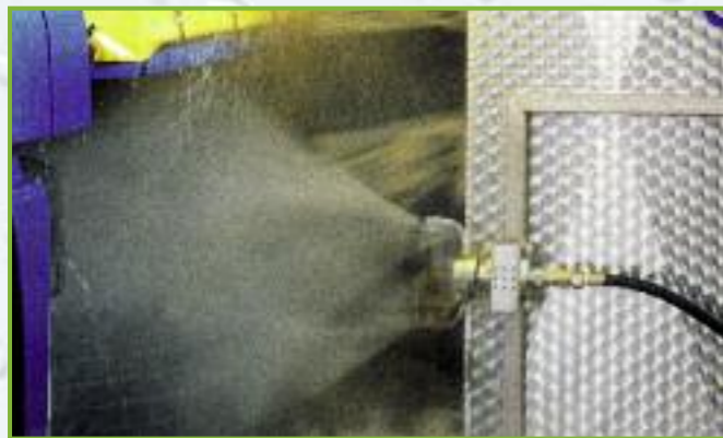
Pump module for chassis and wheel wash.
