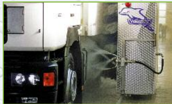
Chassis and wheel wash system connected to a truck washing machine.
