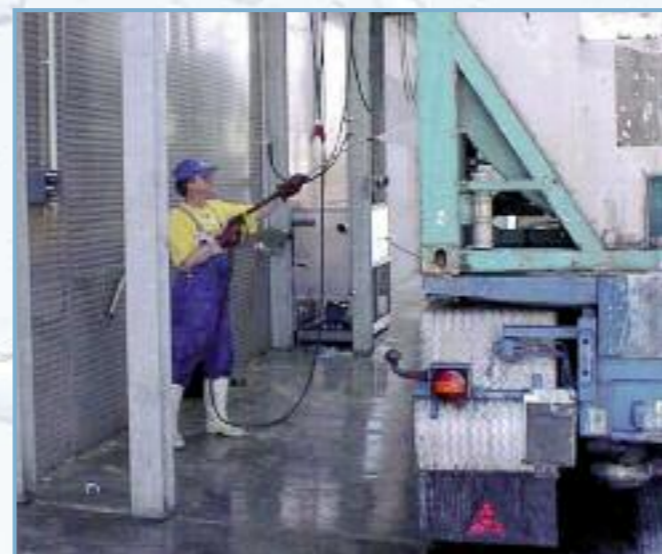
High pressure cleaning with the hand gun of manhole cover, hoses and valves.
