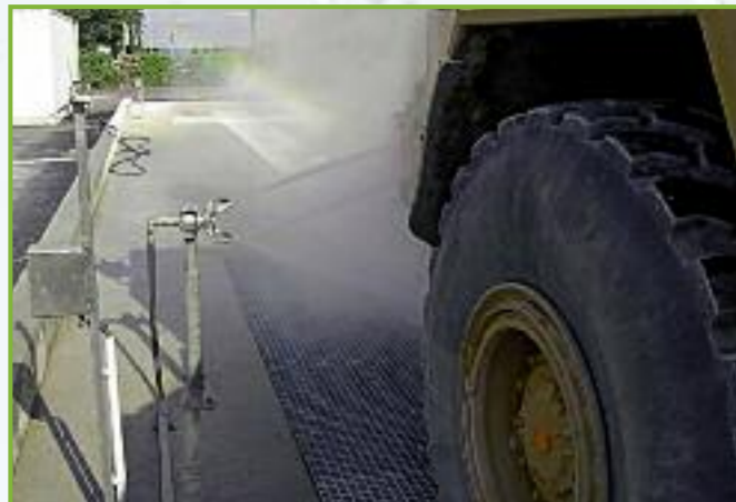
Chassis and frame washing.
